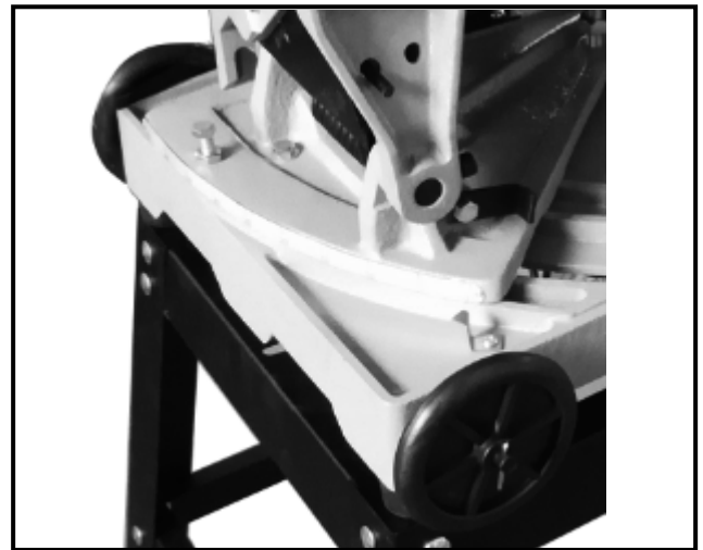
Figure-6 Installing two wheels onto the base
